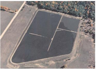
Figure 14. Dredged sediment disposal cell.
