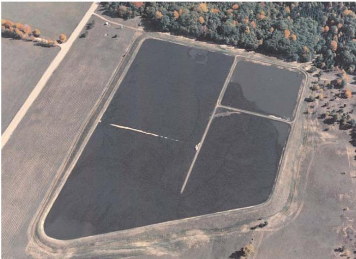
**Figure 14. Dredged sediment disposal cell.**
